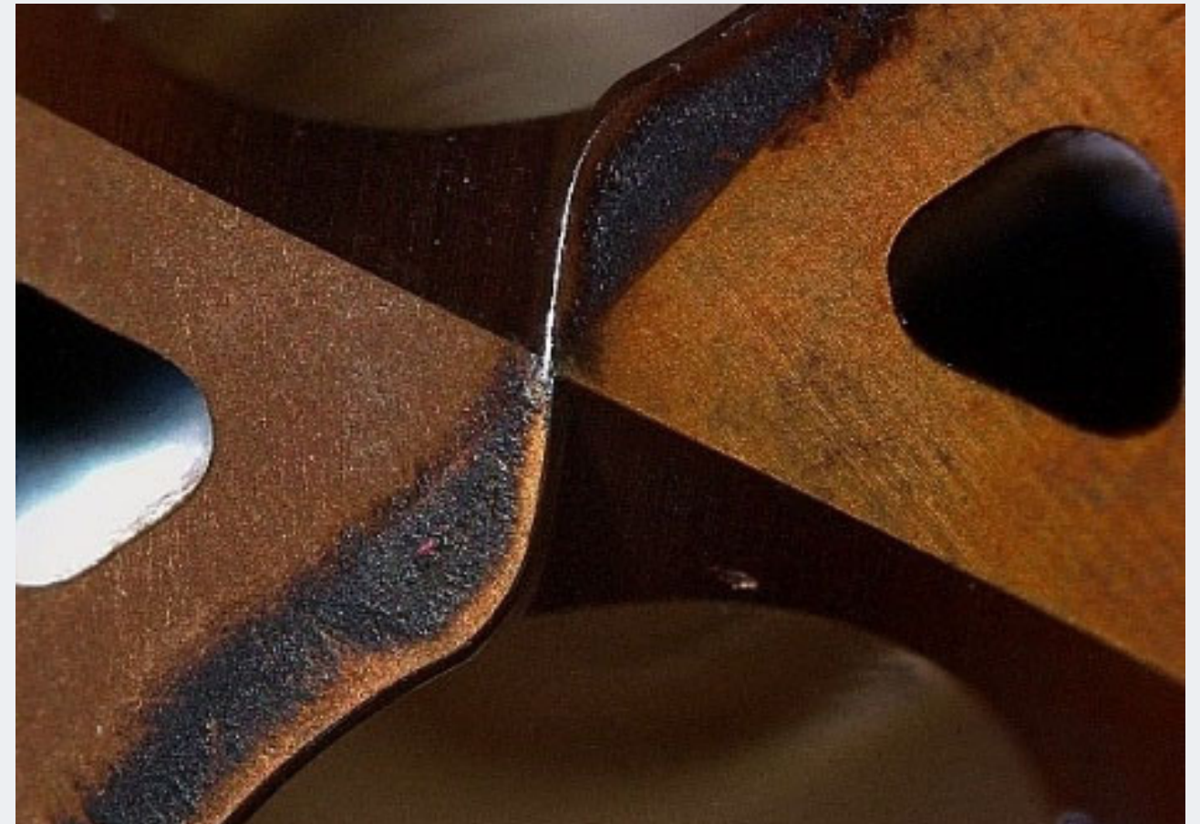
Fig 1 - Example of drill after cutting 20 holes
