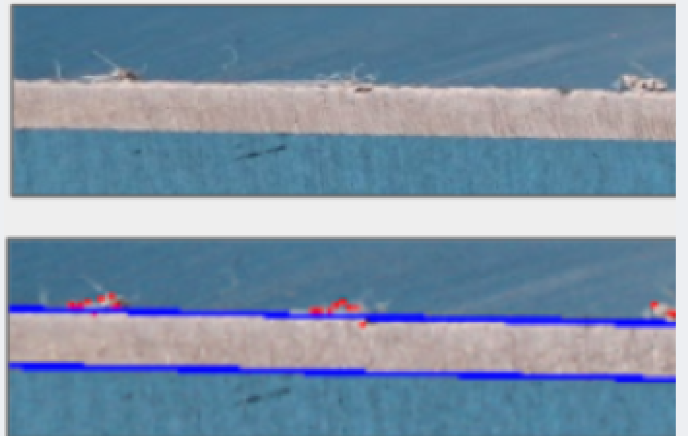
Fig 2 - Close up of unclean burr, detected in red
