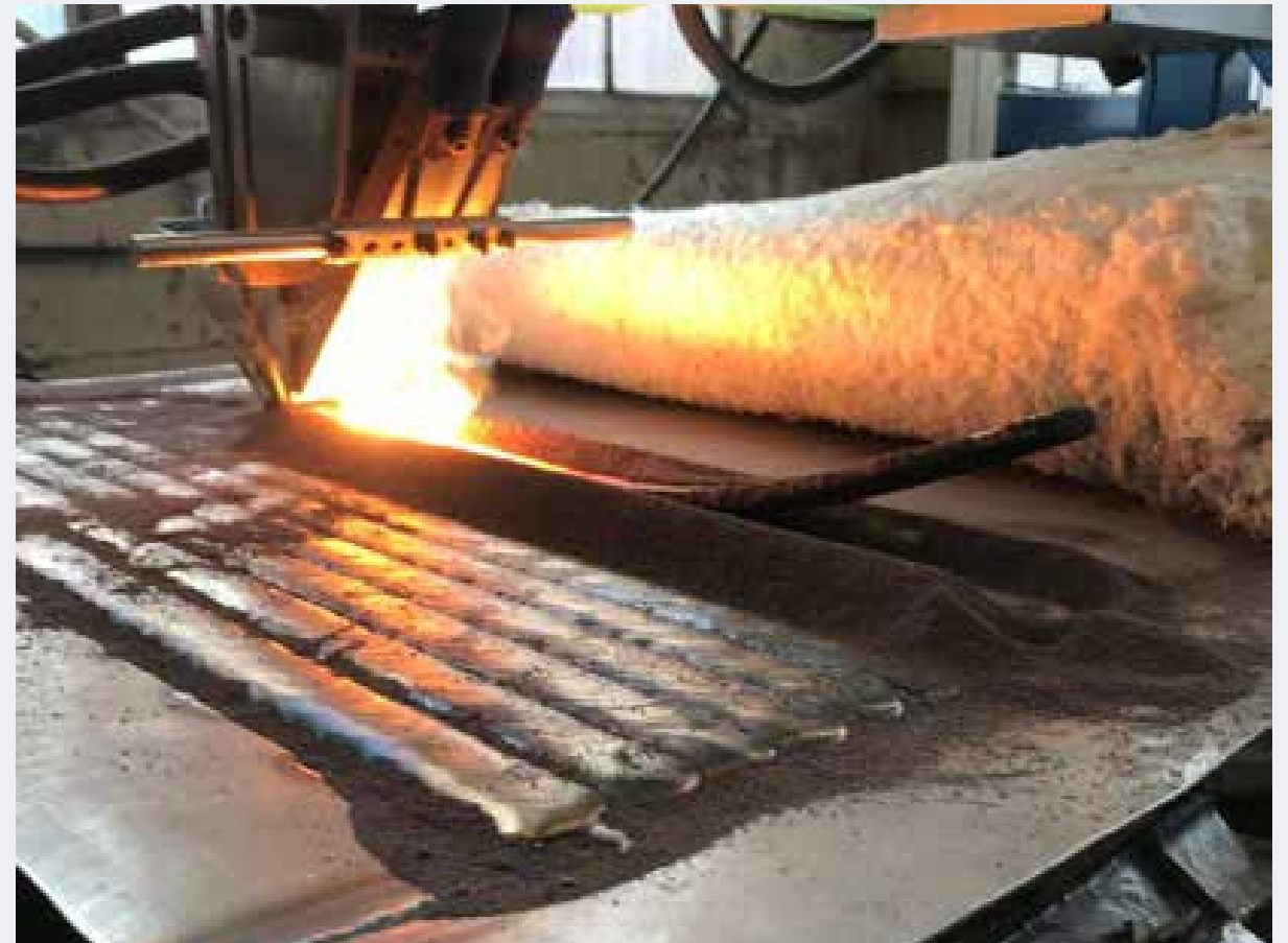
Fig. 1 - ESS Process showing multiple passes on full-scale plate. Slag is shown peeling from metal.
