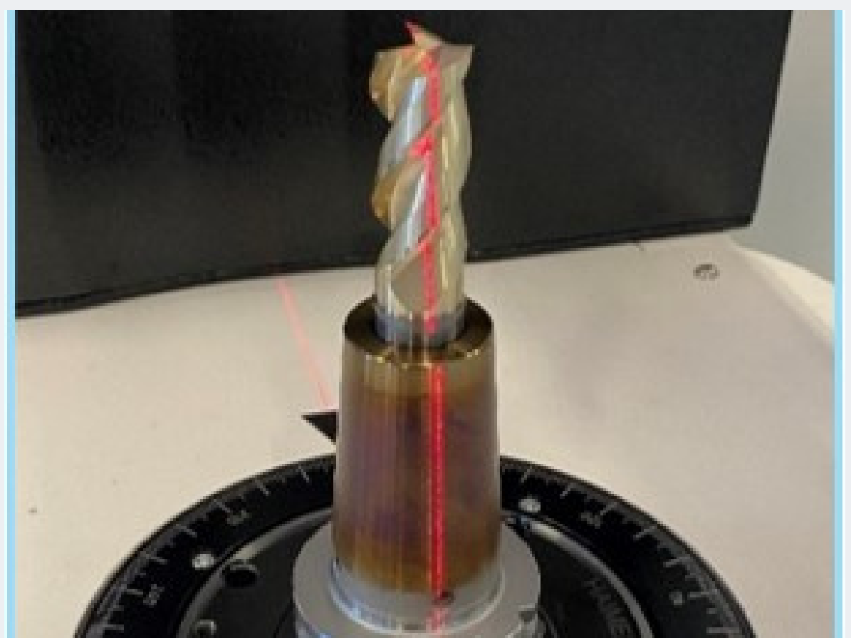
Figure 2 - Cutting tool being balanced with a laser.
